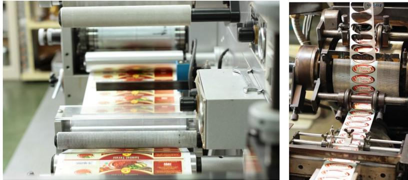
(Gambar Kiri) STEP 2: Proses Finishing. (Gambar Kanan) STEP 3: Proses Plong
